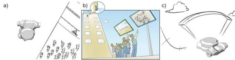
Figure 1. (a) Climbing an outdoor wall, (b) live video from an onboard camera is transmitted to a screen at ground level, (c) flying under remote control.
