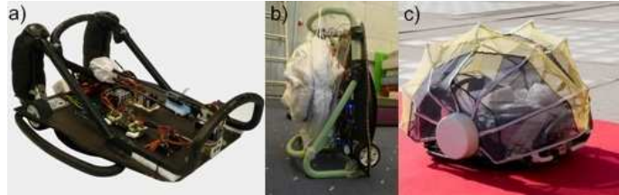
Figure 7. (a) The robot. (b) With folded paraglider. (c) With design shell.
