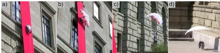
Figure 9. The four key stages of climbing, transition, flying, and landing. The hanging cord visible in (a) and (b) is a lightweight safety cord to constrain the maximum range of the flying robot.
